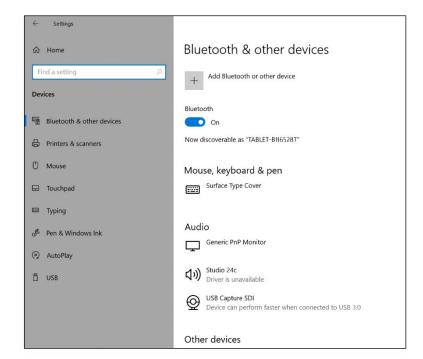
Here you will find the camera unde the Audio heading. The camera has a name containing the string: **'USB Capture SDI'**
