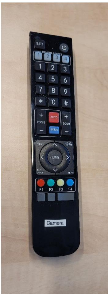
It is possible to control the pointing and zooming of the camera. For this there is a remote control on the speaker desk. Please leave this control on the speaker desk at all times, especially when you leave the room after the class has ended.
